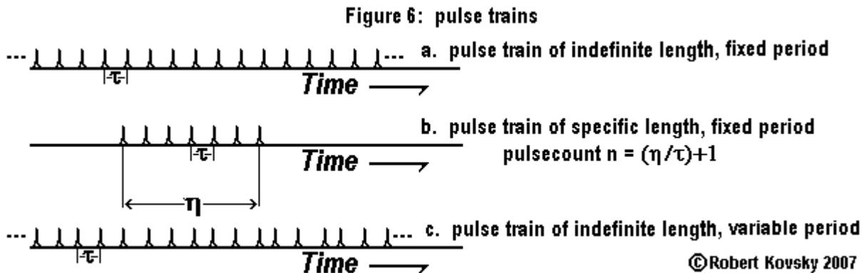
The pulse train of specific length in Figure 6.b has a specific duration, denoted by  $\eta$ , as well as a fixed period,  $\tau$ , between pulses. The number of pulses in a pulse train of specific length is called the **pulsecount** and is denoted by  $n$ :  $n=(\eta/\tau)+1$ . A single pulse (as in Figure 1) is an extreme example of a pulse train, where  $\eta=0$  and the pulsecount = 1.
