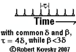
Figure 2.a shows a simple assembly – called a “4-cycle” – made up of four identical primal timing devices. A projection from one primal timing device becomes a projection onto another primal timing device. The timing devices have a common  $\delta$  and  $\beta$ . During operations, each primal timing device produces pulses in a steady stream, called a *pulse train*, shown in Figure 2.b.
