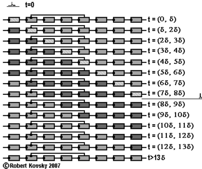
In sum, the assembly generates a pulse train like that shown in Figure 4 when  $\beta < 3\delta$ . On the other hand, for a similar single input pulse, the assembly produces only a single pulse output when  $\beta > 3\delta$ .
