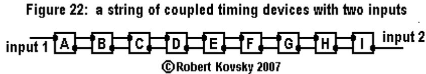
Using the typographical notation to represent activity of a string of coupled timing devices with  $\beta = 2\delta$ , Figure 23 shows that a pulse incident through input 1 and a pulse incident through input 2 will cancel or annihilate each other. Such cancellation does not depend on details of timing, only on the pulsecount. To illustrate this fact, the pulse through input 1 occurs at  $t=0$  and the pulse through input 2 occurs at  $t=\delta$ , so that cancellation occurs away from the center.
