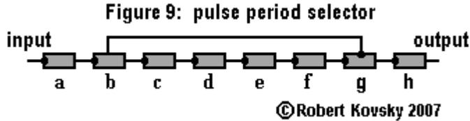
The *pulse period selector* shown in Figure 8 passes or blocks a pulse train according to the period between pulses. Its function is like a bandpass filter in electronics that passes or blocks a periodic signal, e.g., a sine wave, according to the frequency.
