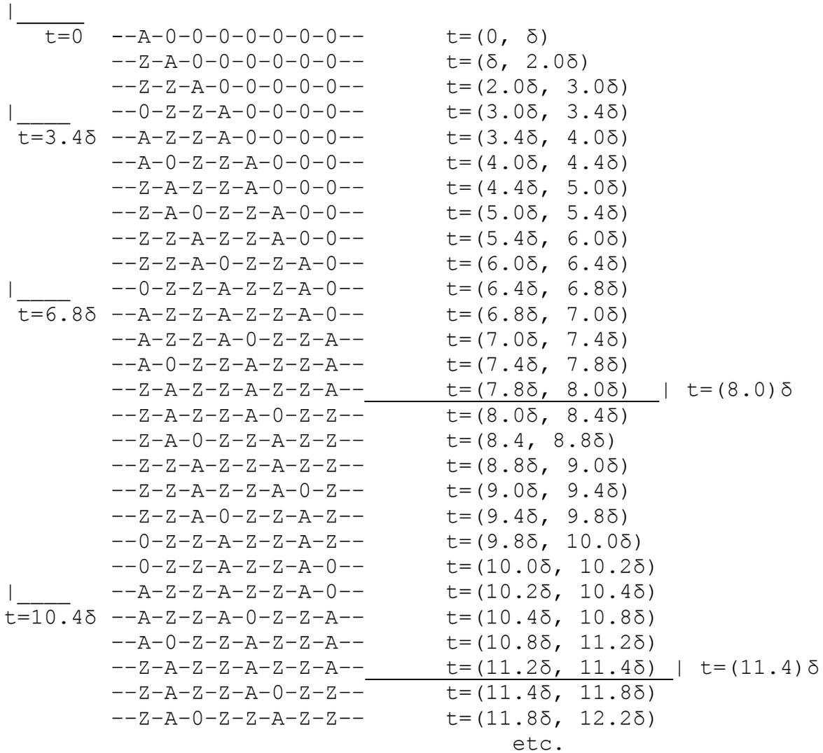
Pulse progress charts are similar to charts used to track activities of cellular automata (See, e.g., S. Wolfram, *A New Kind of Science*); but cellular automata are based on an invariant clock tick and do not participate in phase changes like timing devices.
