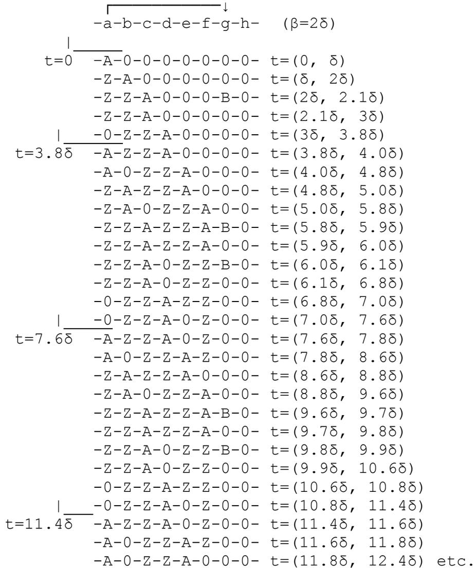
Examination shows that a pulse train will pass through the pulse period selector if the period between pulses,  $\tau$  in the pulse train, is within limits defined as  $(4.0\delta - \xi) < \tau < (4.0\delta + \xi)$ . Hence, the pulse period selector resembles a bandpass filter in electronics.
