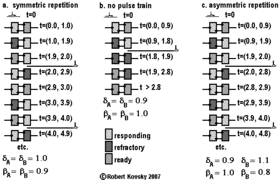
Figure 17.c shows how variations in timing intervals control pulse patterns: start with the coupled timing devices in operation with the timing intervals shown in Figure 17.b. Leaving timing device A untouched, change the timing intervals of timing device B to those shown in Figure 17.c to get the new kind of response, "asymmetric repetition," that can produce a pulse train identical to that shown in Figure 17.a.
