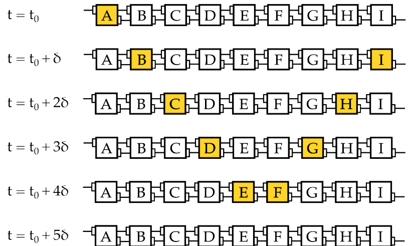
Fig. 19: pulse cancellation in a bi-directional array of timing devices, \beta > \delta
